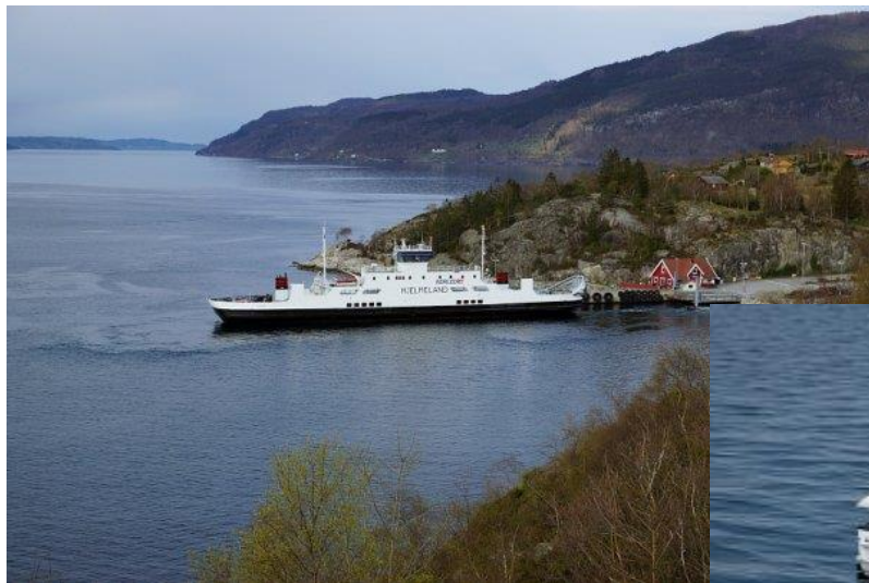
Hydrogen-electric car ferry. Foto: Helge Stikbakke/ Statens vegvesen
